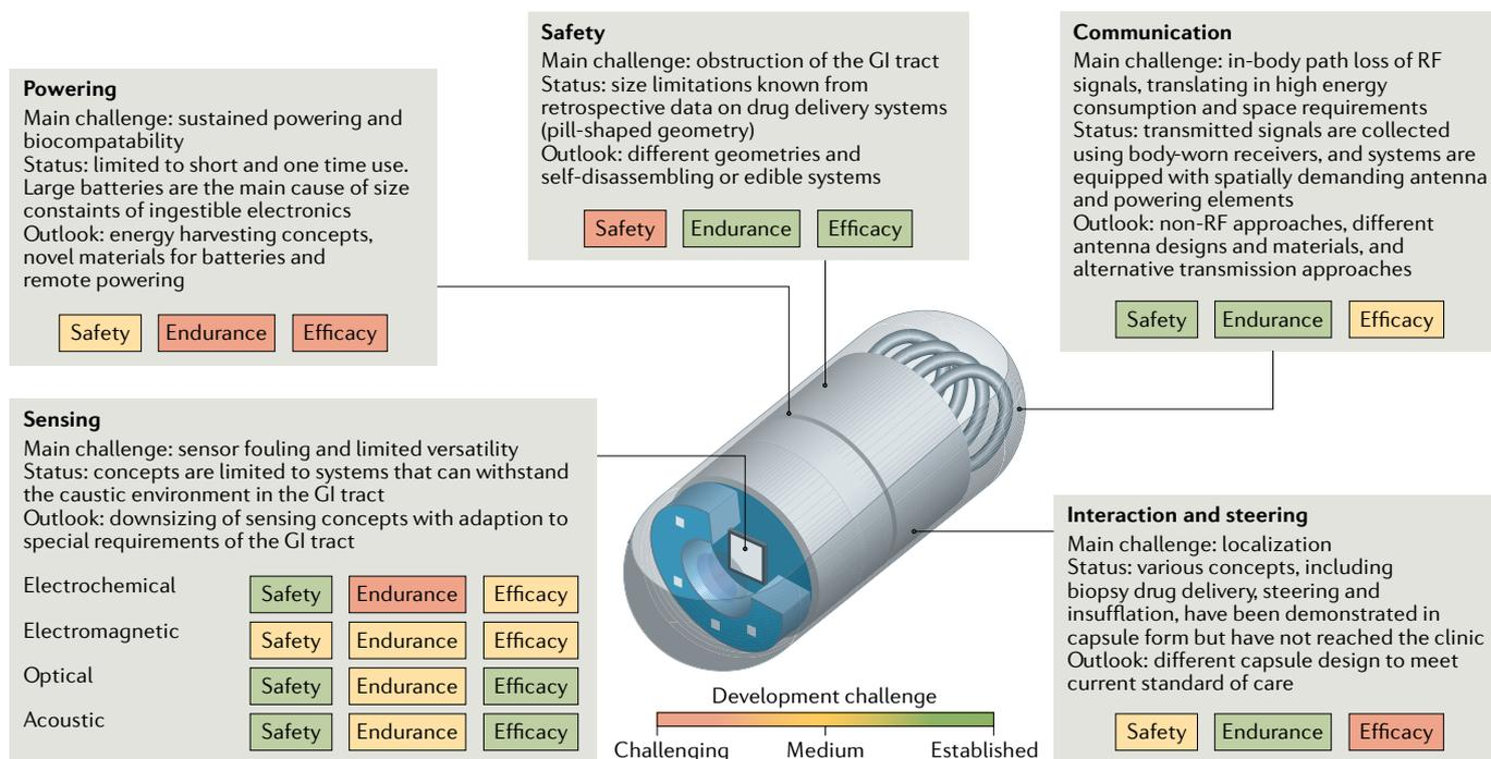
Fig. 7 | **Major challenges for ingestible electronics.** Main challenges for powering, sensing, communication, safety and tissue interactions are illustrated using a standard ingestible capsule design. GI, gastrointestinal; RF, radio frequency.
