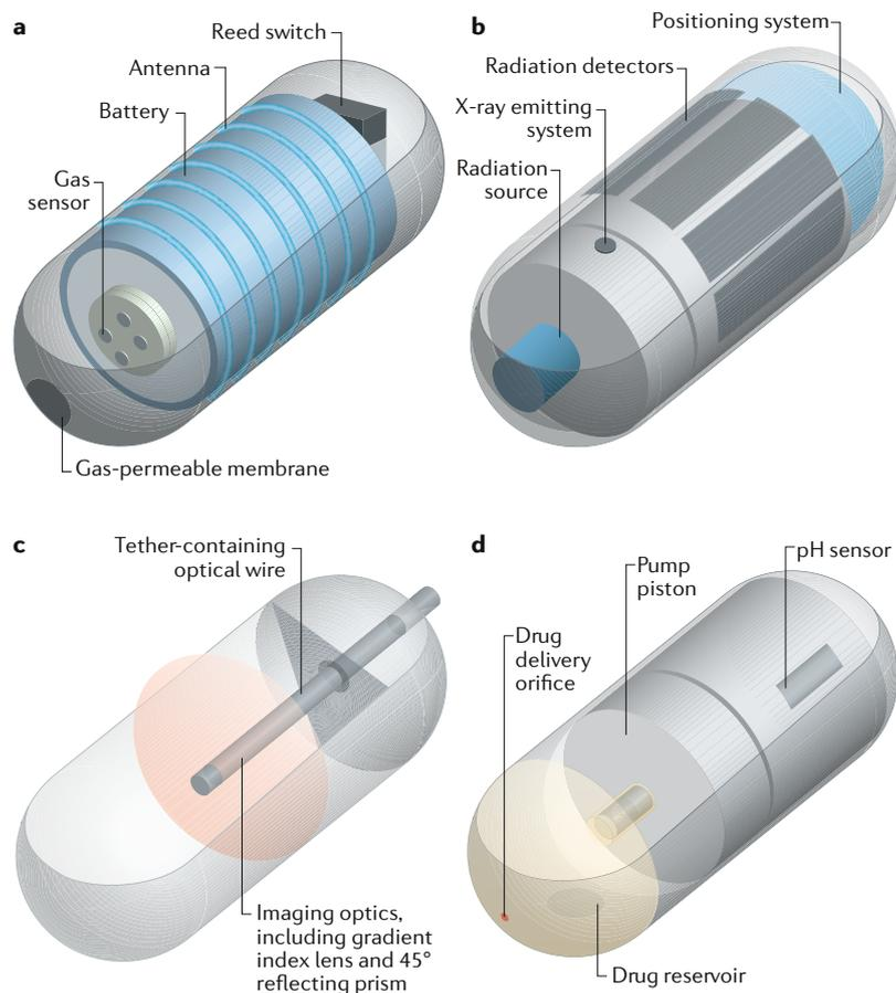
**Fig. 4 | Technologies for ingestible electronics.** **a** | Gas-sensing capsule. **b** | X-ray scanning capsule. **c** | Optical coherence tomography. **d** | IntelliCap for drug delivery. Panel **a** is adapted from REF.<sup>95</sup>, Springer Nature Limited. Panel **b** is adapted with permission from Check-Cap. Panel **c** is adapted from REF.<sup>142</sup>, Springer Nature Limited. Panel **d** is adapted from REF.<sup>158</sup>, CC BY license.
